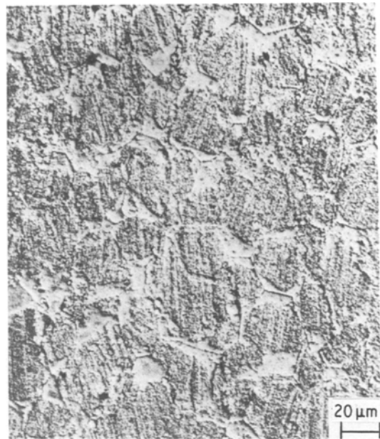
Figure 12 Precipitate free zones (PFZs) observed near grain boundaries in a Mg alloy [98].
